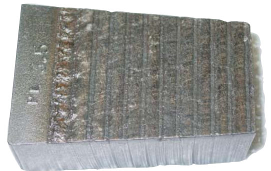
Tough stuff. JET Technologies' process grew one-eighth of an inch of titanium nitride inside a U.S. Army tank center guide made of a titanium alloy. Tests showed a significant increase in wear resistance.
